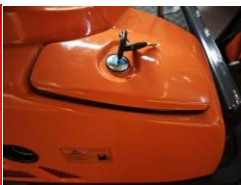
hydraulic oi Tank location
